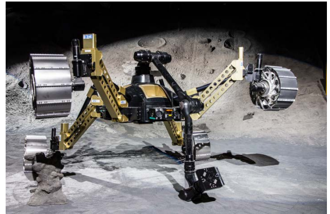
Sherpa's Manipulator is strong enough to support the robot when two wheels are lifted off the ground.
