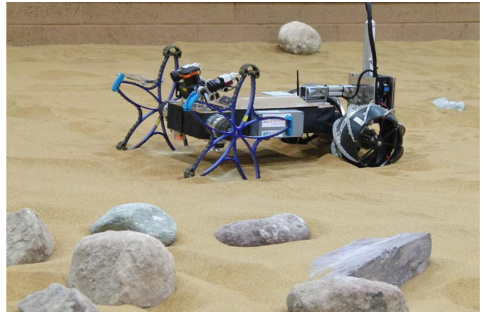
Coyote II equipped with full sensor suite including its soil sensor system payload developed by Surrey Space Center
