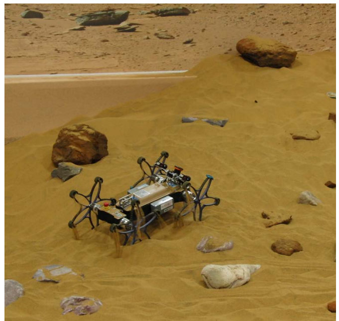
Coyote II with tilted rear axis, equipped with four hybrid legged-wheels
