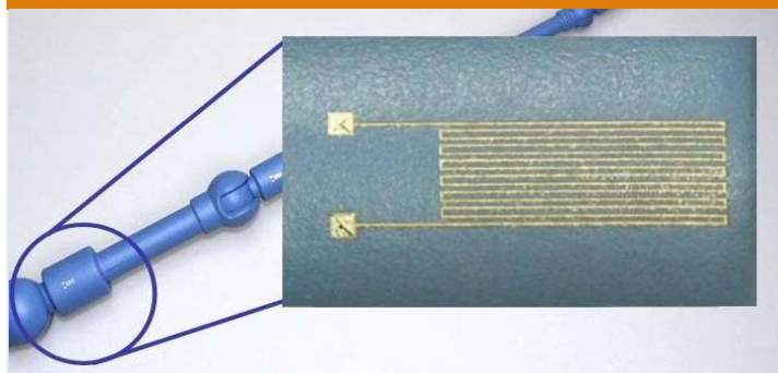
Fabrication procedures allow a high freedom to print miniaturized sensor elements. The procedures permit a precise shaping on arbitrary substrates with a resolution > 10 \mu\text{m} .
