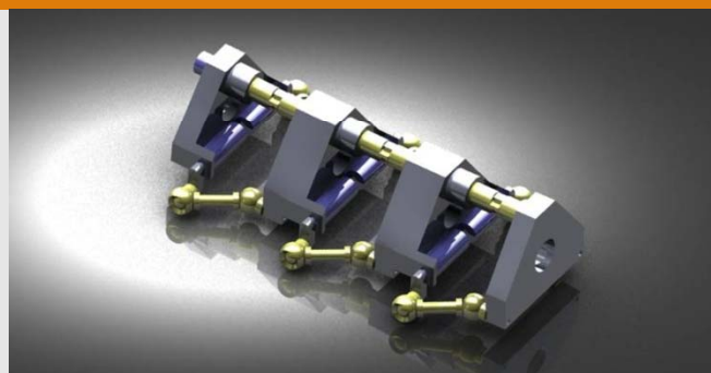
CAD drawing of a first concept of an artificial spine. The single elements of the spine are built modularly to allow a serial arrangement of the elements. Wires can run through the center of the spine.
