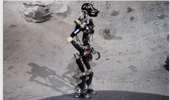
The transition into a bipedal posture allows the robot to use its arms for alternative tasks.
