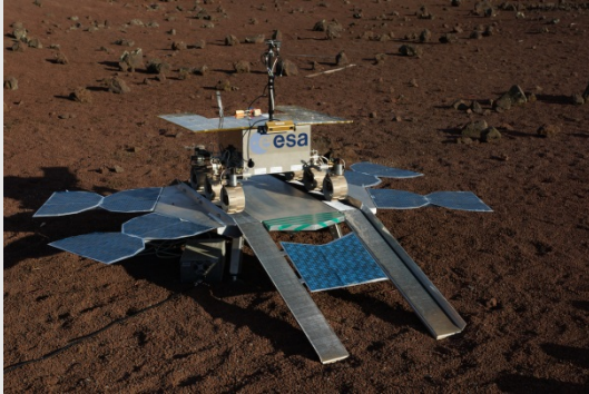
The ExoMars Testing Rover (ExoTeR) is ESA's half-scale reproduction of the ExoMars rover. ExoTeR is the testing platform for the SARGON activity. (Photo: Martin Azkarate, ESA, HESpace)
