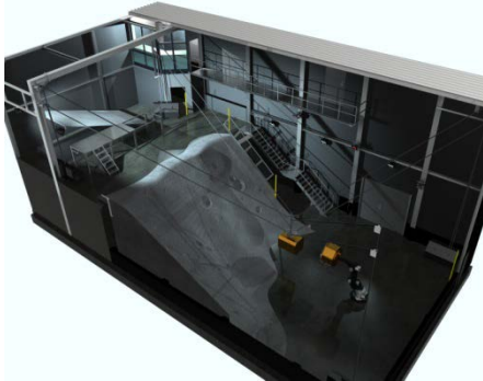
Computer graphic of the test facility for mobile robots (DFKI Space Exploration Hall)
