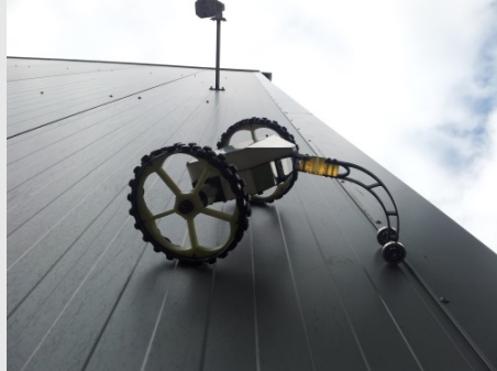
An ultra-light magnetic crawler for the inspection of cargo holds and ship hulls.
