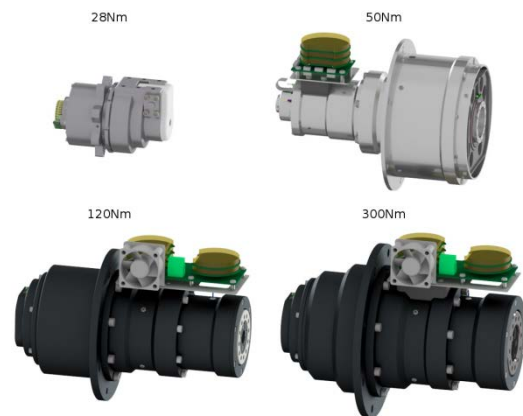
Set of actuators designed in the project
