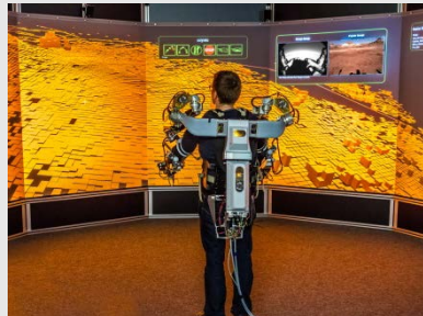
Control of Coyote III by using the exoskeleton in the Virtual Reality Lab, Bremen
