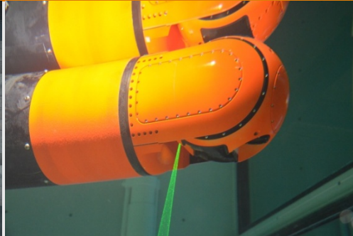
Fig.2: Inspection unit (HD-Kamera, Structured Light System, Multibeam Profiling Sonar)
