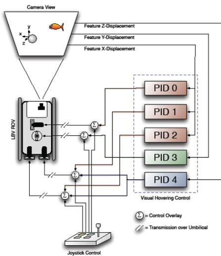
Fig. 1: Structure of the ROV Hovering system controller
