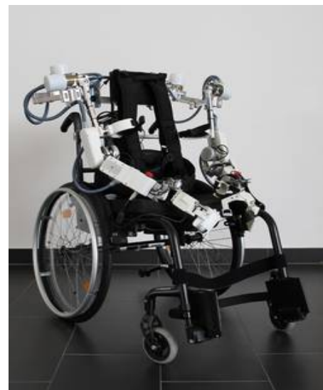
The active dual arm exoskeleton in its resting state
