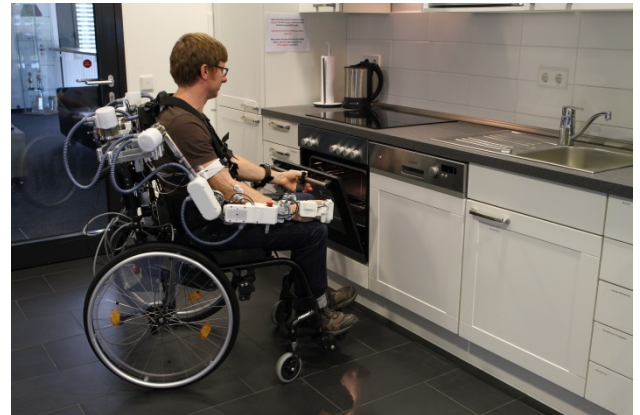
The system covers the entire kinematics of the human arm
