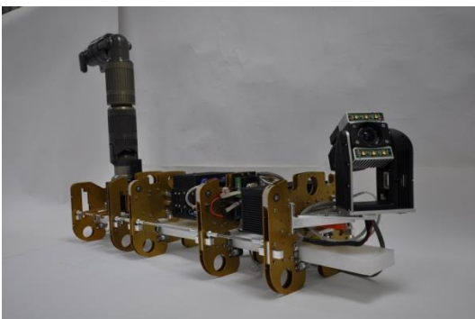
ARTIS Demonstrator with 3D rail guidance capability
