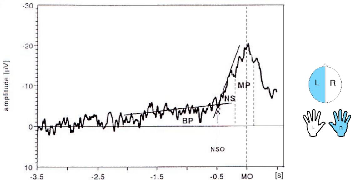
**Fig1. Pre-movement MRCPs.** Averaged EEG recording from electrode C1 (left side of the scalp) preceding right hand index movement. The slow negative slope associated to the early BP is named in the picture as BP. NS indicates the late BP and NSO its onset, which is located about 500ms before movement onset (MO). MP indicates the steep increase in negativity which occurs immediately before movement-onset<sup>6</sup>.
