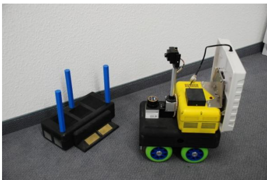
A docking station provides 24/7 operational time. The recharging process is initialized autonomously by the robot.
