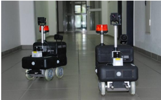
The SentryBot systems are able to navigate autonomously indoors.
