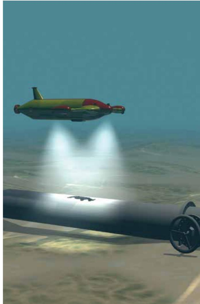
Pipeline tracking in the deep sea by means of intelligent robots
