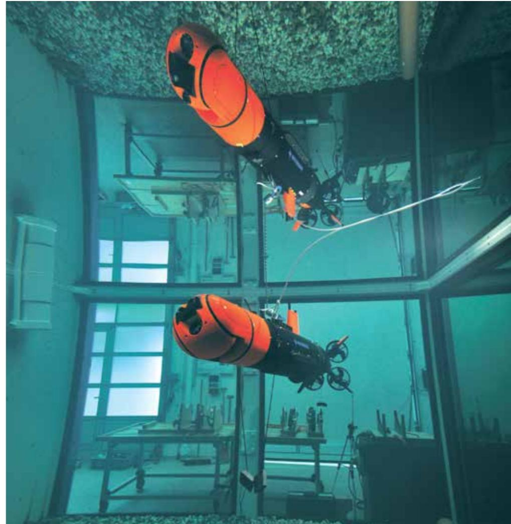
Diving in the glass tank: an AUV built by ATLAS Elektronik with integrated DFKI technology
