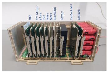
The heart of the rover, the configurable EPS is equipped with a backplane and allows to quickly move technologies to be tested in a real system.
