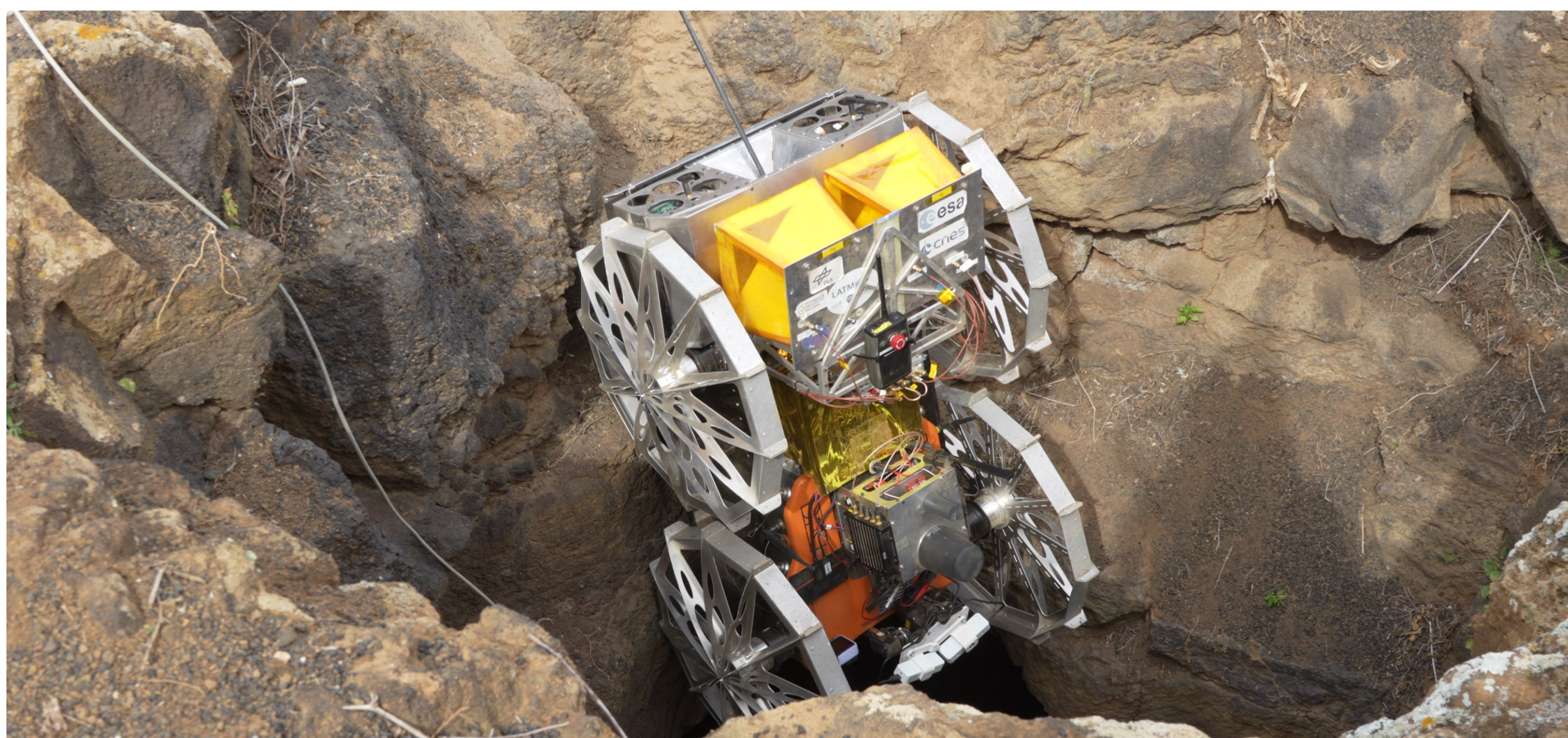
Rappelling into a lava tube with rugged metallic wheels, tethering module, ground penetrating radar and a computing payload (Photo: Meltem Fischer)
