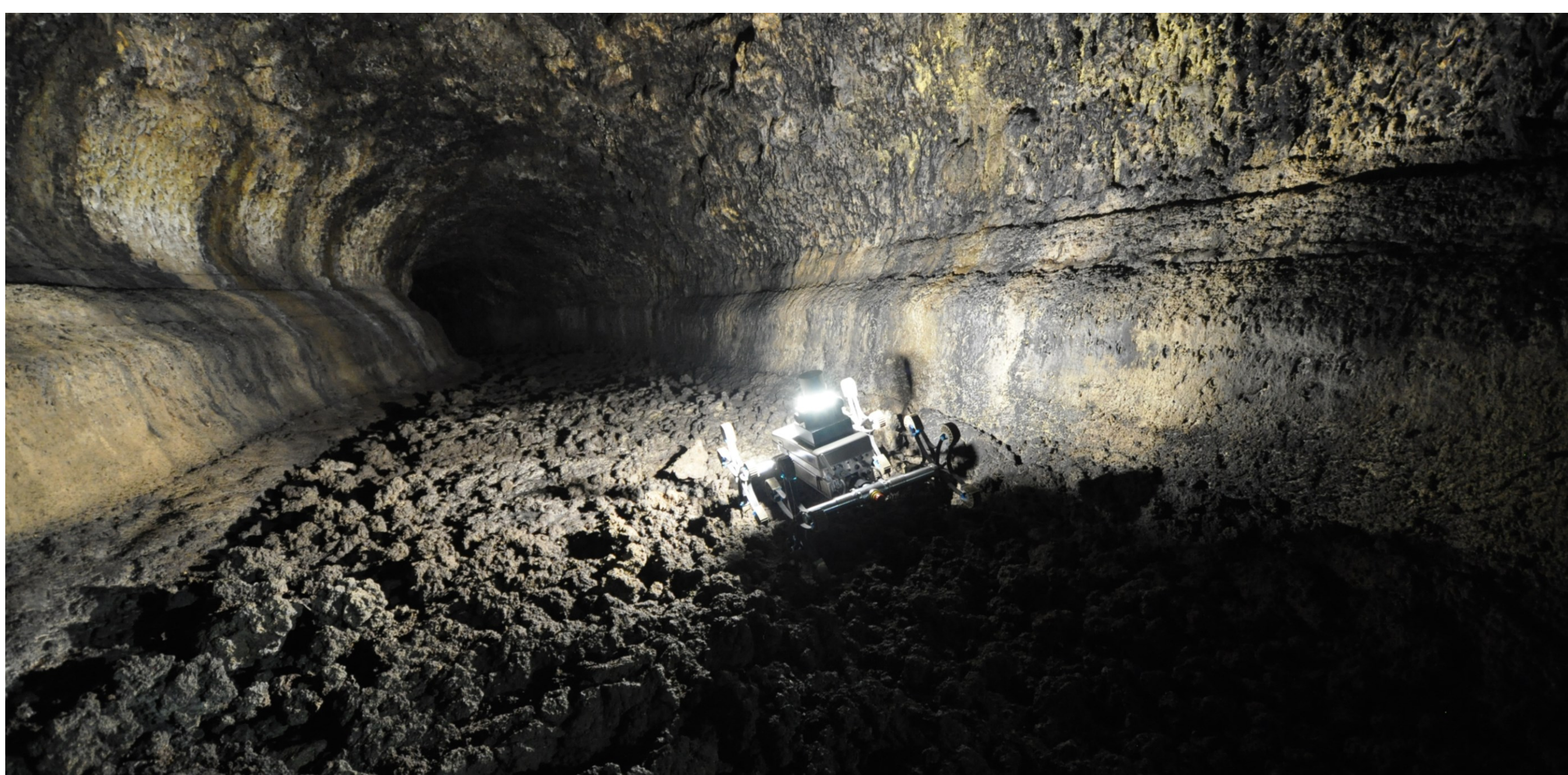
Asguard v4 navigates through steep slopes and harsh surfaces in a lava tube. (Photo: Raúl Domínguez, DFKI GmbH)
