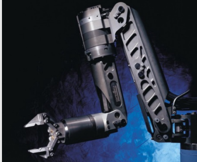
Orion7P Schilling Robotics manipulator (Quelle: Schilling Robotics)
