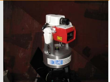
An optical laser tracker is used for the localization of the individual robots of the Minoas fleet
