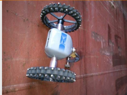
DFKI prototype for an ultra-light magnetic crawler for the inspection of cargo holds and ship hulls
