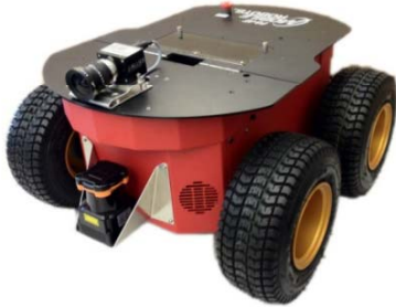
Several robots of the type Pioneer P3-AT will be used for exploration and for the localization of the lunar modules which will be collected by Amparo.
