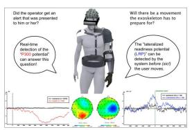
aBRI – adaptive Brain Reading: Single trial EEG analysis for operator state prediction
