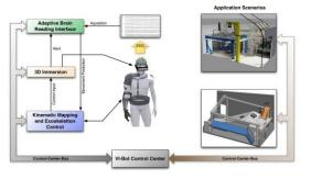
Cooperation of VI-Bot project components, here: exoskeleton, visualization, and aBRI as well as both demonstration scenarios.
