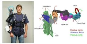
Photo and concept design of the actuated Exoskeleton-Arm.
