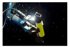
The Schilling deep-sea robot arm, which is used in the CManipulator project
